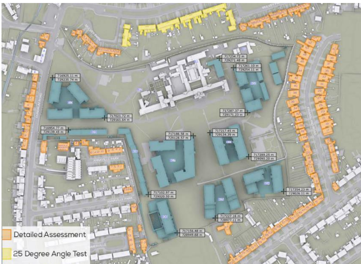
Figure 9: Daylight, Sunlight, Overshadowing Image from GIA Report
