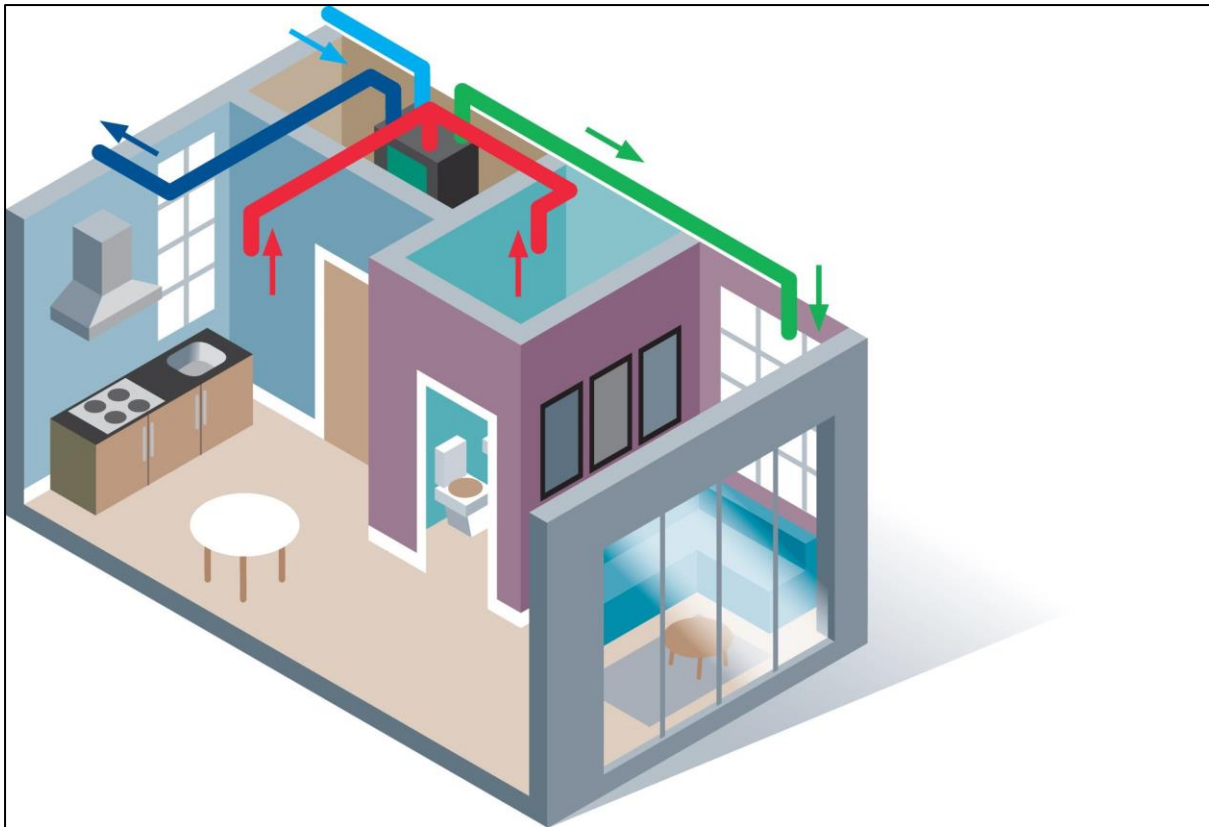
Figure 4: Mechanical Ventilation System
